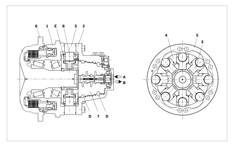
Hydraulic motors of the type MCR-T are radial piston motors with front case mounting and flanged shaft. They are specially designed for track drive applications and are primarily used as drive motors on skid-steer loaders and compact track loaders.
