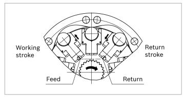
The number of working and return strokes corresponds to the number of lobes on the cam multiplied by number of pistons in the cylinder block.
