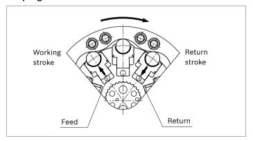
The number of working and return strokes corresponds to the number of lobes on the cam multiplied by number of pistons in the cylinder block.
