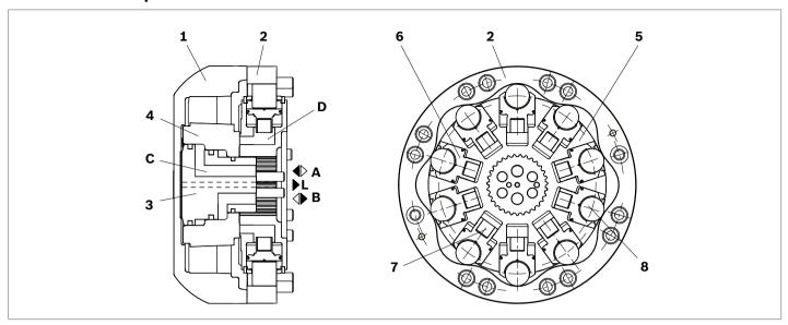
Hydraulic motor type MCR-R is a radial piston motor with a rotating case designed for installation on a vehicle axle to provide hydraulic drive to its wheel.
